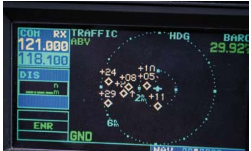
Just another busy day at Ardmore. The two aircraft on the left showing +24 (2400 feet above) and +29 are departing from Runway 05 at Auckland International Airport.
