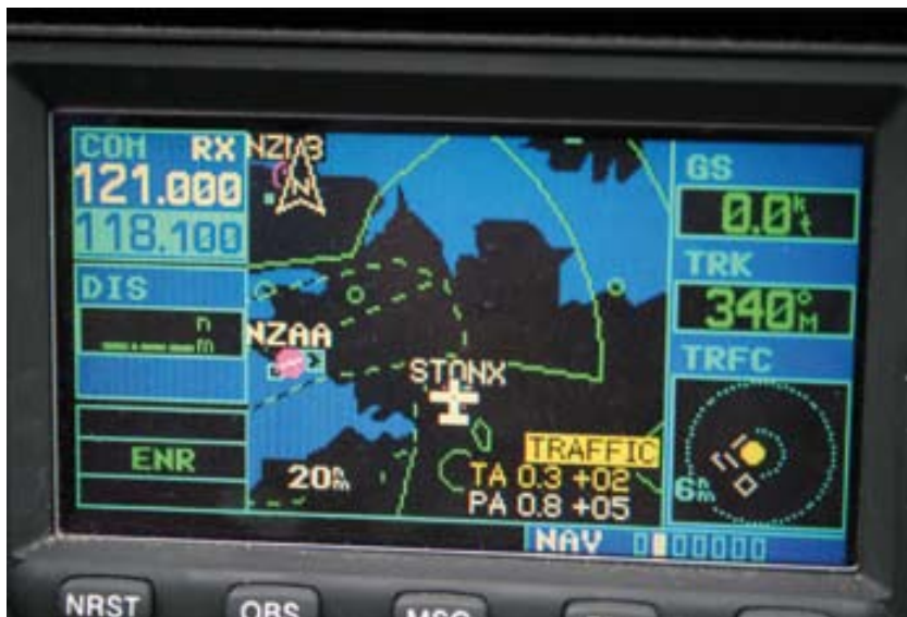
The Map page, showing a Traffic Advisory (TA), which is traffic within 500 feet altitude and not diverging. The Proximity Advisory (PA) is traffic within 500 feet altitude but not as high a risk as a TA. On the bottom right is a thumbnail of the traffic's position.
