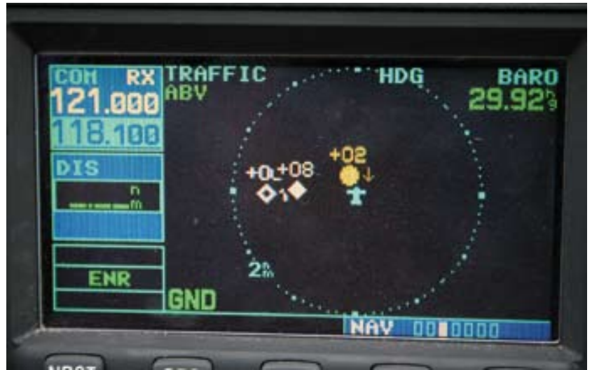
Not a sight you ever want to see. This is another aircraft a very short distance away, 200 feet above, but descending.
